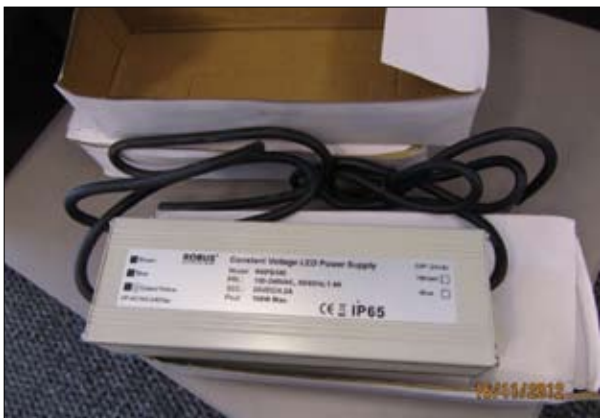
Fig 17 Unapproved power supply – North Parramatta
