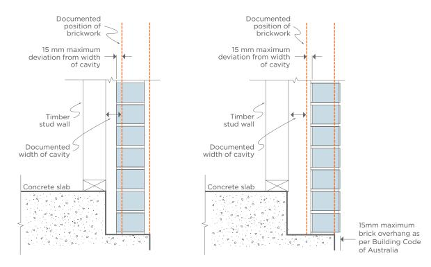
L Note: Refer to the Building Code of Australia for minimum cavity width.
