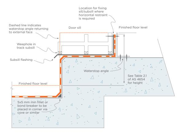
**DIAGRAM 14.06B** TYPICAL DETAIL OF A MEMBRANE AT A WALL OPENING WHERE INTERNAL AND EXTERNAL FLOOR FINISHES DO NOT ALLOW FOR AN UPTURN
